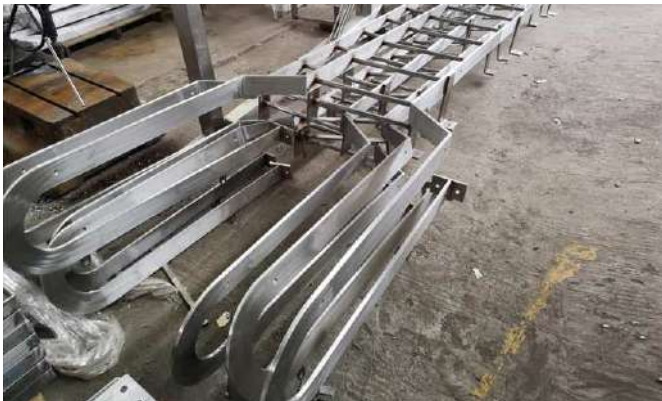
水務署貓梯 (WSD 7.3 H) Cat Ladder of Water Supplies Department (WSD 7.3 H)
